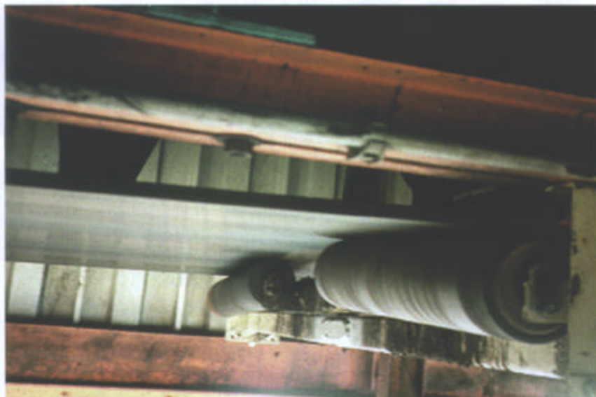
A self-adjusting, three-roll idler adds extra support to the belt and helps prevent misalignment.
