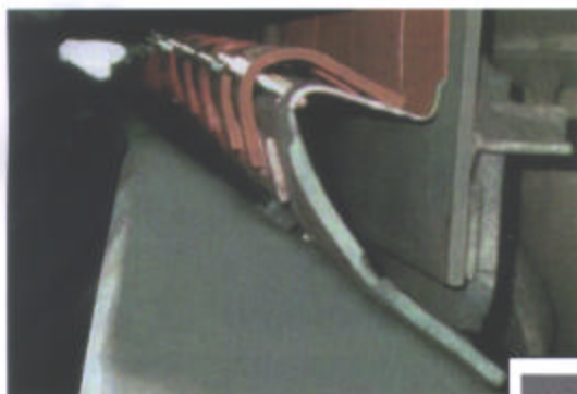
A good conveyor belt sealing system will prevent spillage problems.
