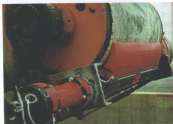
There are many various accessories to conveyor belts that will improve its performance, including the belt cleaner pictured here.
