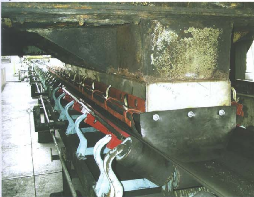
A Flexiskirt sealing system and a Simplicity slider bed installed at a conveyor load area.
