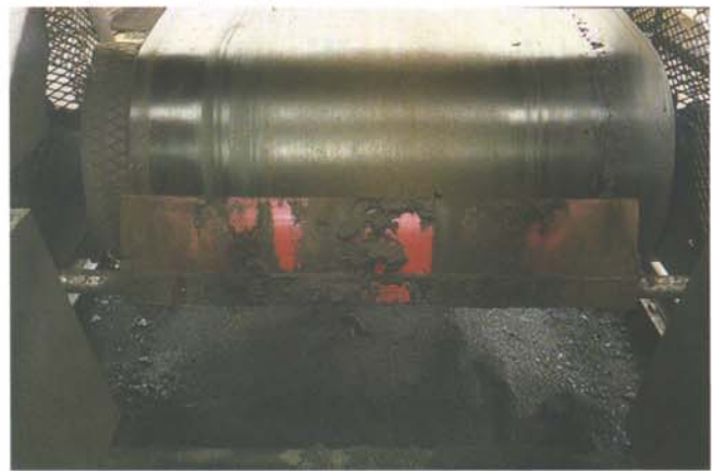
A Gordon Saber primary belt cleaner installed on a conveyor head pulley.
